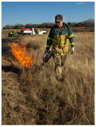
The most widely used ignition device is a drip torch. Drip torches use a mixture of diesel and gasoline. A mixture of 50:50 diesel to gasoline works very well for temperatures ranging from 35 F to 75 F. When temperatures are higher than this, a mixture of 60:40 or 70:30 diesel to gasoline is recommended to reduce the volatility of the gasoline and to help the torch operate properly. (Photos courtesy: J. Weir top and bottom left, J. Bradley top right, T. Johnson bottom right)
