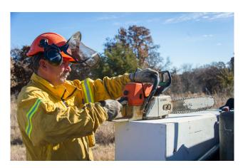
When using a chainsaw, safety should be your top priority. Chainsaw operators should wear full protective gear. Care should be taken when operating the chainsaw near hot spots on the tree due to the air movement created by the saw, which can cause flames to flare-up injuring the operator or damaging the saw. (Photo courtesy T. Johnson)
